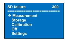
If the SD-card is removed during the writing of data an error "SD failure 300" will occur. The number at the right will count down. It is possible to reinsert the SD-card while the counter is still active. The data will still be saved. Not reinserting the SD-card will result in data loss.
