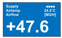
The plus sign indicates that an air inlet is being measured. It is also indicated as SUPPLY on the upper left of the display.
