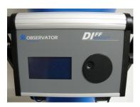
The DIFF can be switched on by pushing in the <u>middle</u> of the scroll button. The recess in the scroll button is intended for scrolling through the menu.
