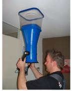
The **AT-242** is required for measuring supply and exhaust vents in residential housing. This light hood simply slides over the top of the Diff and doesn't require any additional tightening.
